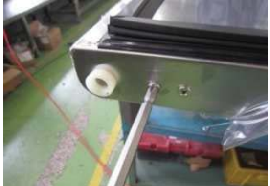
G. Assemble stopper plate in original positions.
