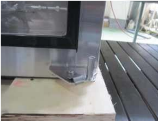
G. Assemble stopper plate in original positions.
